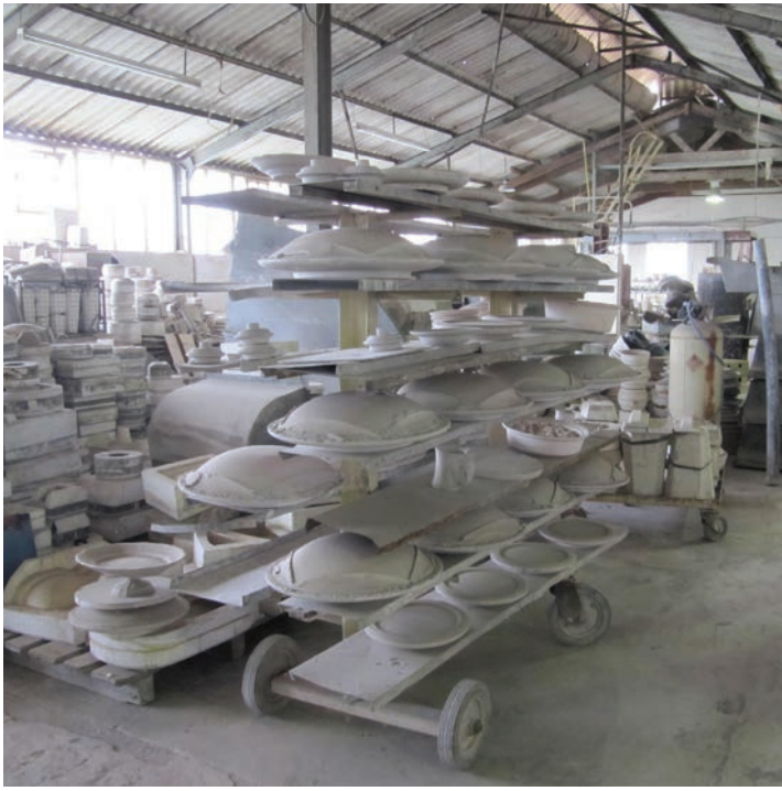
Opposite page: left to right 1. Filter press at Oude Kaap factory 2. Semi automatic flat ware roller machine This page: 3. Flat ware moulds, Oude Kaap factory
