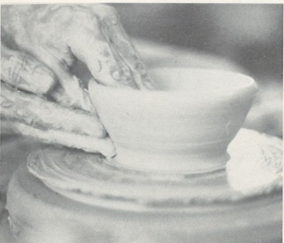
B5 Once again the next step is an important one as here the right hand pushes in to form the bowl foot while the left hand supported by the right steadies the clay and keeps the pot on center.
