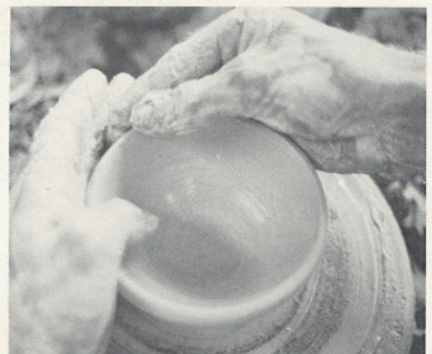
B4 The left hand continues keeping the pot steady and on center while the thumb and forefinger of the right hand form the rim.
