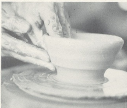
B6 The clay is now pulled up in one steady movement.
