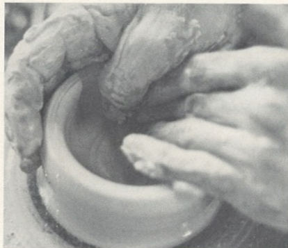
C3 Once open squeeze the clay between the thumb and fingers of the right hand and pull up.
