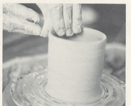
C8 Using the thumb and forefinger of the left hand, steadied by the right hand, form the rim by pressing slightly down and out. This will give a nice generous rim, gently flaired and ideal for drinking from.
