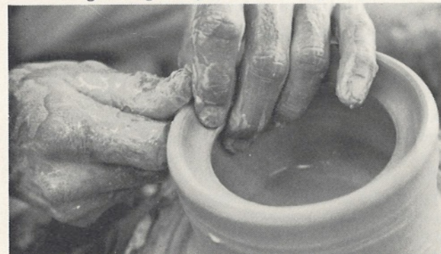
6. Note the right thumb and index knuckle forming the rim and keeping the pot on centre.
