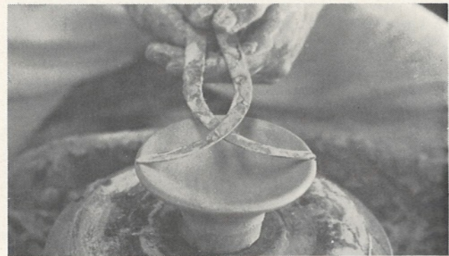
6. Measure the outer edge to fit. If necessary repeat steps 3 and 5 to adjust.
