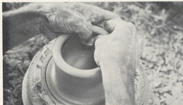
4. To pull up squeeze the clay between the thumb and fingers of the right hand, the left hand steadies the pot. Pull the pot about halfway up leaving enough clay to form the galley.
