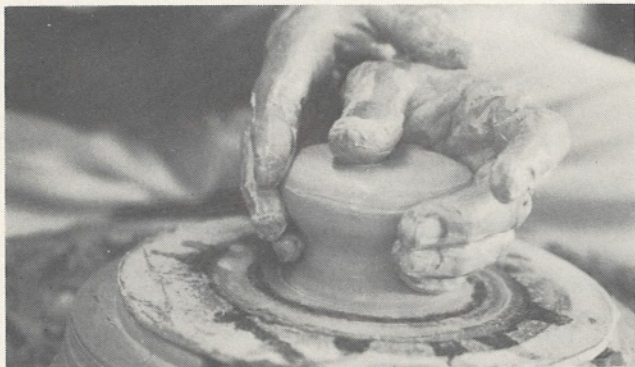
1. For the lid center the clay squeezing in slightly at the base. Notice the braced hands.
