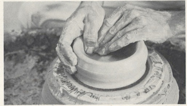
3. Use the fingers of the right hand to steady the clay to the required width.
