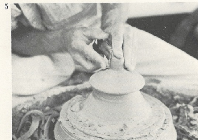
Centre pot firmly on chuck and keep in position with gentle but firm pressure of the left hand (fig. 1), trim off excess clay and form outside of footing. From the centre cut away clay to shape
